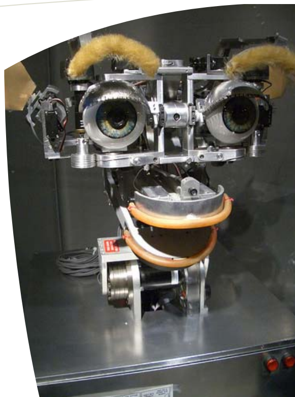
Kismet is an autonomous robot designed for social interactions with humans. Here, he expresses 'surprise' one of 14 discrete facial expressions
